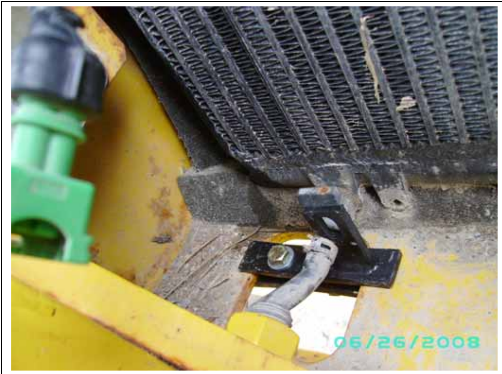
Install lower clamping bracket as shown. (right bracket)
