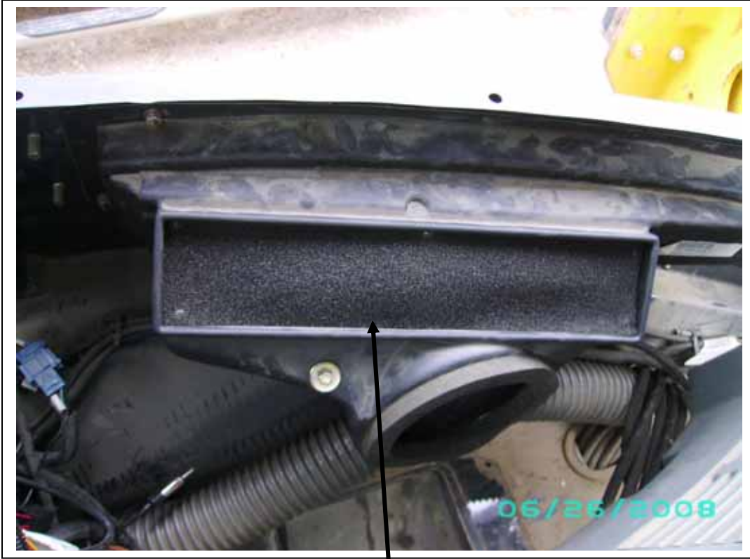
Inside air intake filter installed in plastic air intake box.
