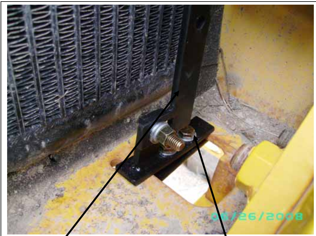
Install lower clamping bracket as shown. (right bracket)
