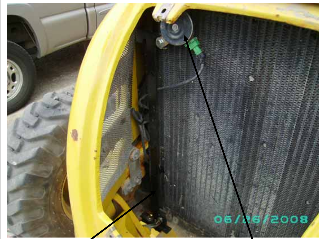
Horn reinstated over right condenser bracket.
