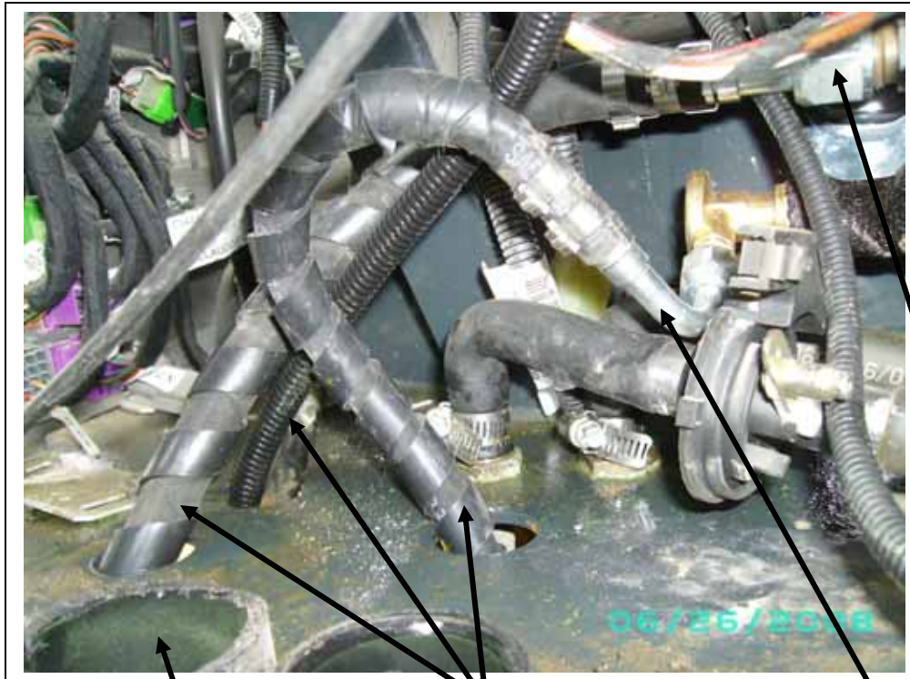
Top cut off 2 1/2" hose adaptor for flex duct to extra louver in cab.
