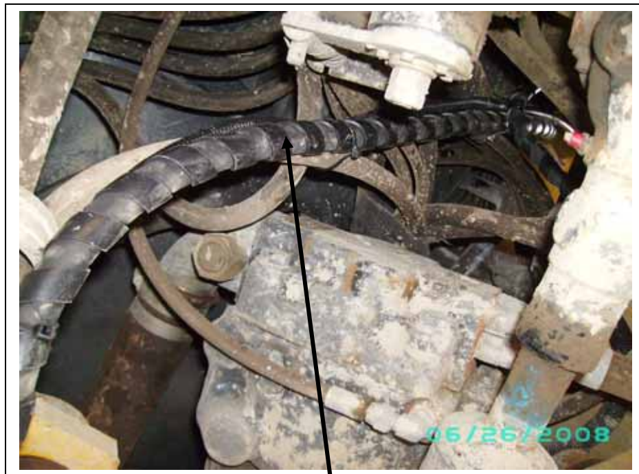
1/2" hose and clutch wire running under the rear engine mount on left side.
