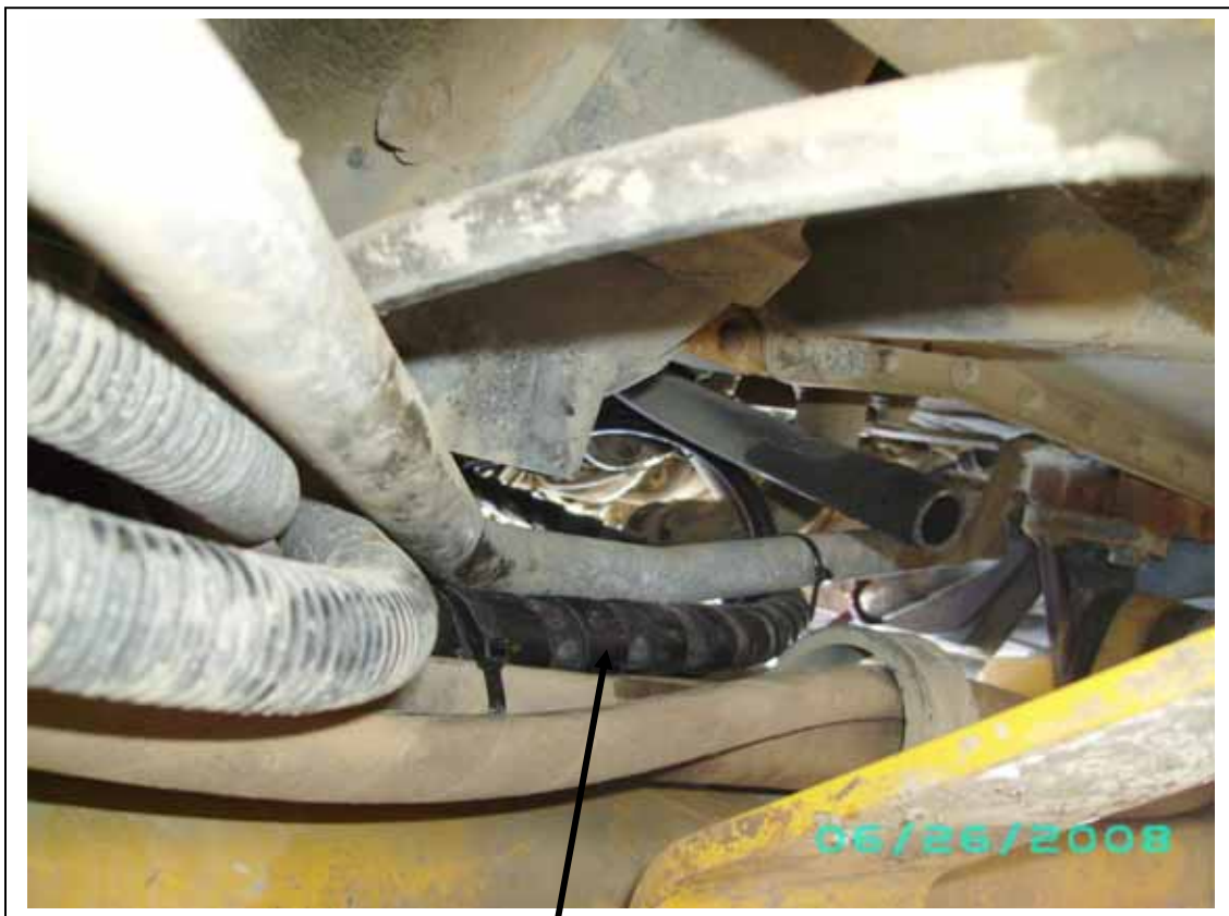
1/2" line and clutch wire running down beside the engine, on the left, and back towards the evaporator.
