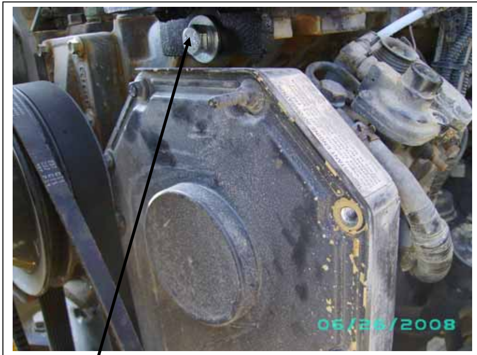
Front fourth bolt on compressor mount bracket
