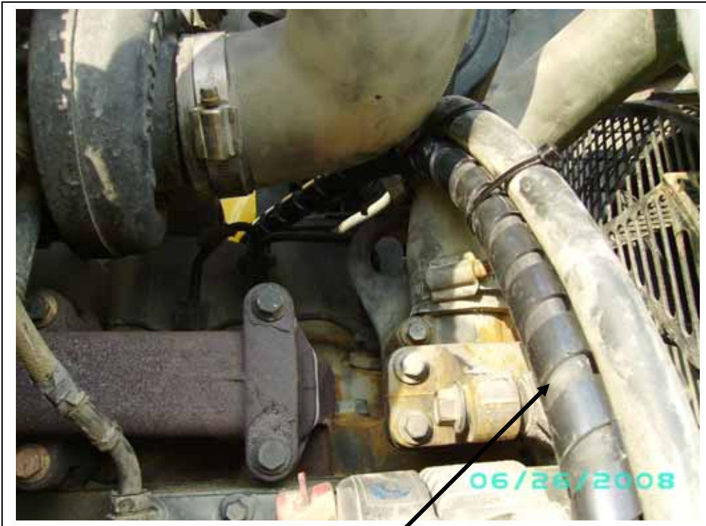
13/32" hose from compressor to condense crossing the top of the engine. Keep tied away from hot exhaust and turbo areas.
