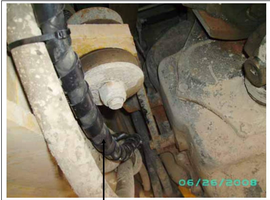
1/2" hose and clutch wire running under the rear engine mount on left side.
