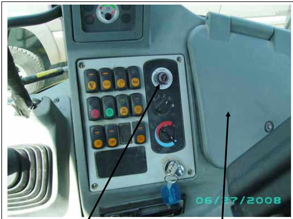
Thermostat in place with switch console reinstalled.
