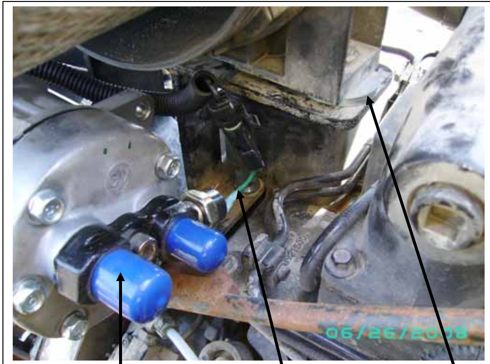
Horizontal O-ring pad fitting c/w binary pressure switch installed on back of compressor.
