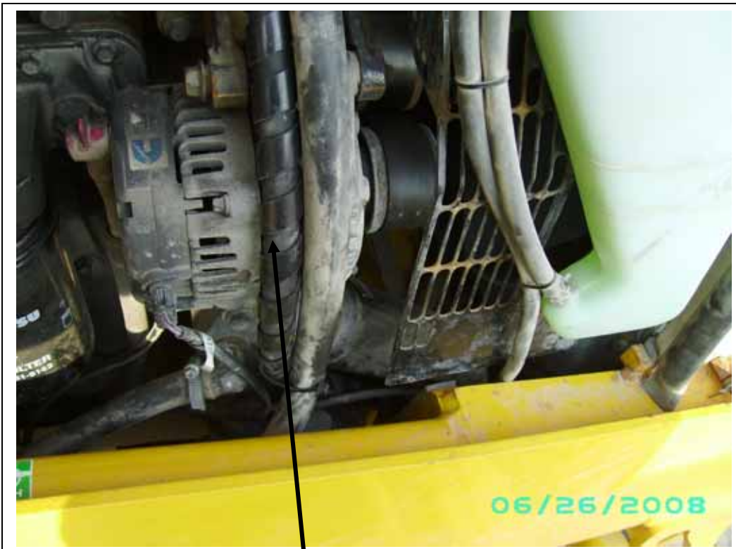
13/32" hose from compressor to condense crossing the top of the engine. Keep tied away from hot exhaust and turbo areas.
