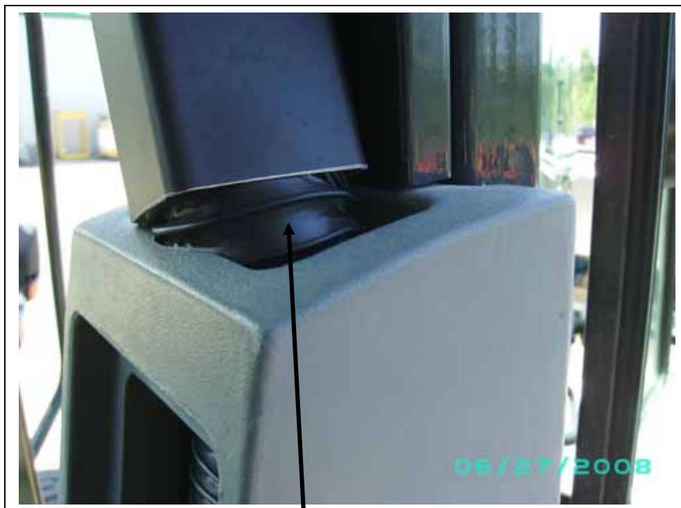
Squeeze 2 1/2" flex duct into the bottom of the square plastic duct provided.
