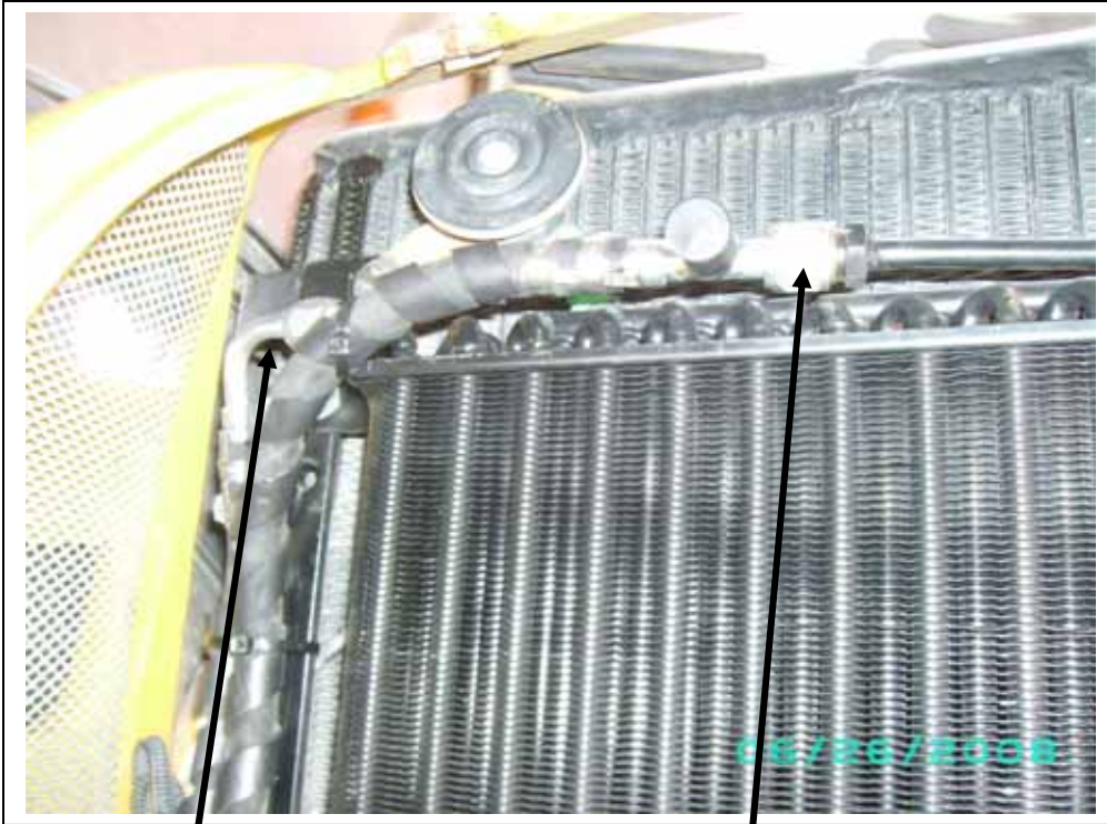
13/32" straight female fitting with 134A access port at the top of the condenser.
