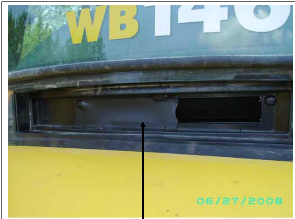
Inside air intake filter installed in plastic air intake box.
