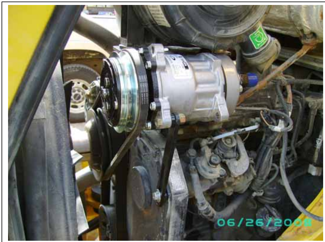
Overall view of the mounted compressor before re-installation of the fan screen.
