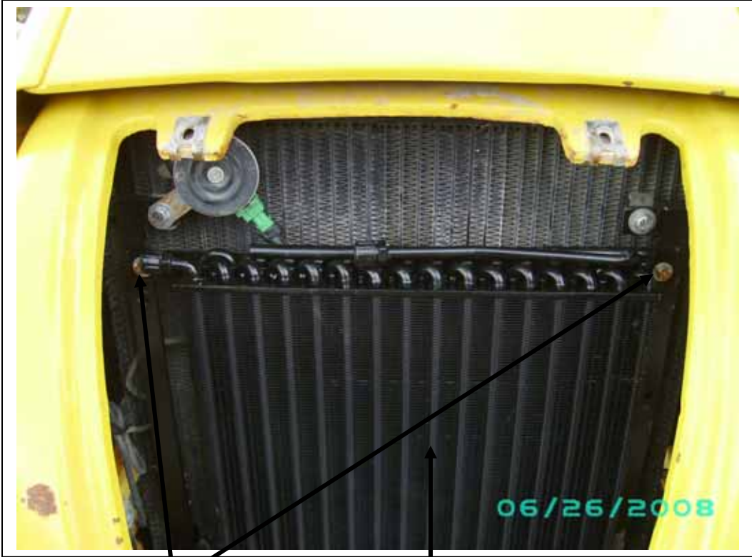
1/4" bolts in threaded holes on condenser bracket.
